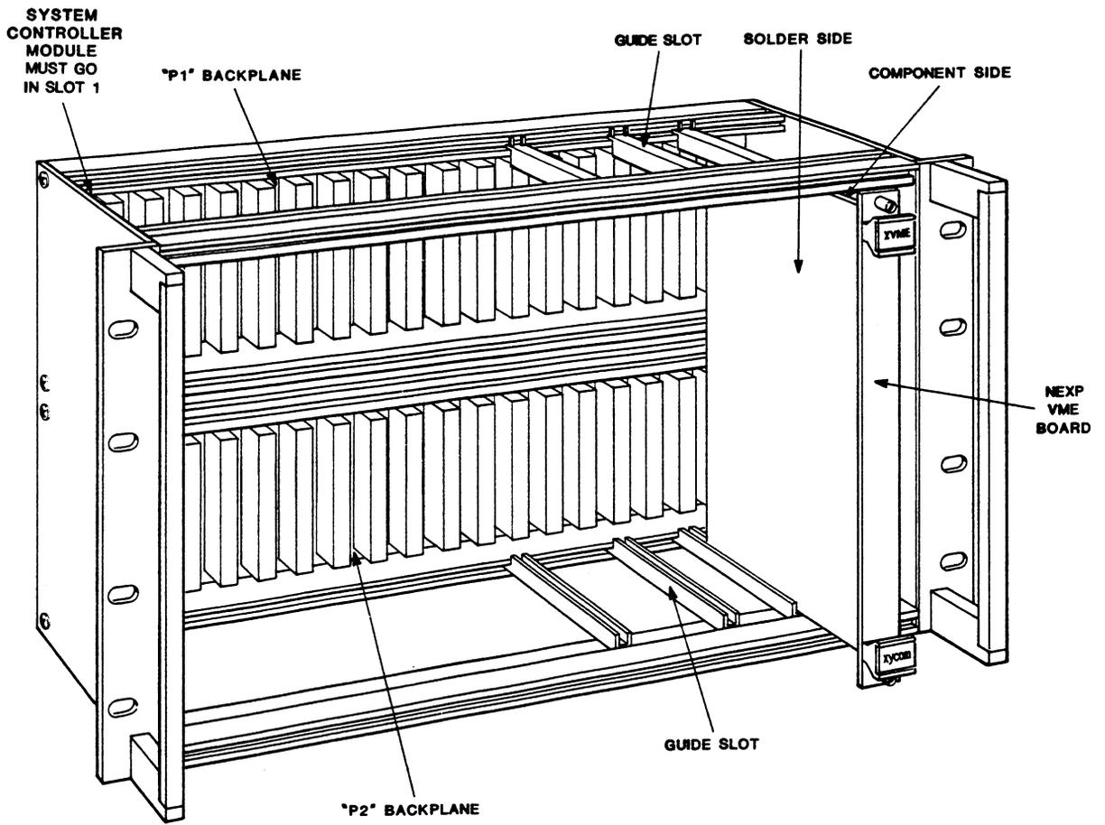
Figure 2-7. VMEbus Chassis
