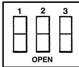
Figure 2-4. Switch Bank 1 Interrupt Level Select Switches
