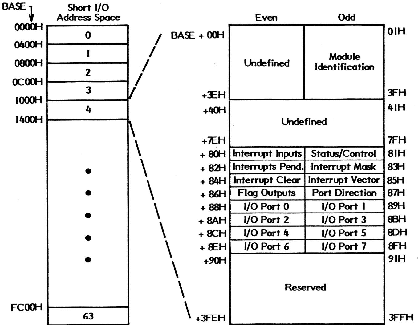
Figure 3-1. The DIO I/O Interface Block and the Short I/O Address Space
