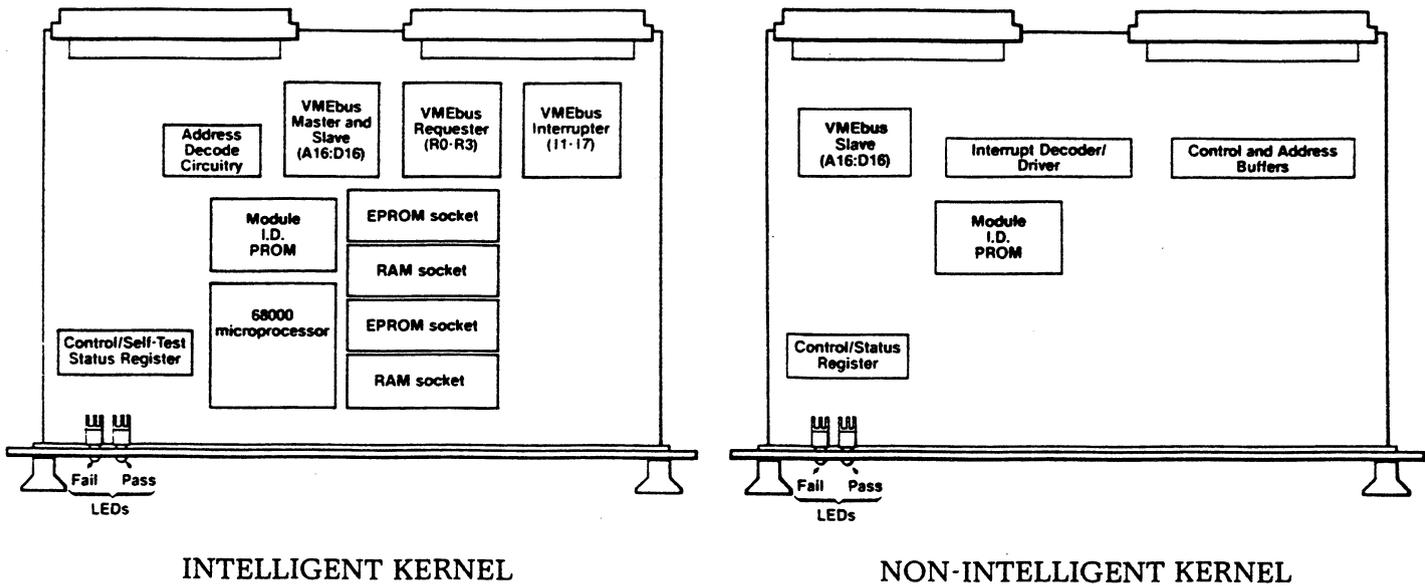
Figure A-5. Intelligent and Non-Intelligent Kernels
