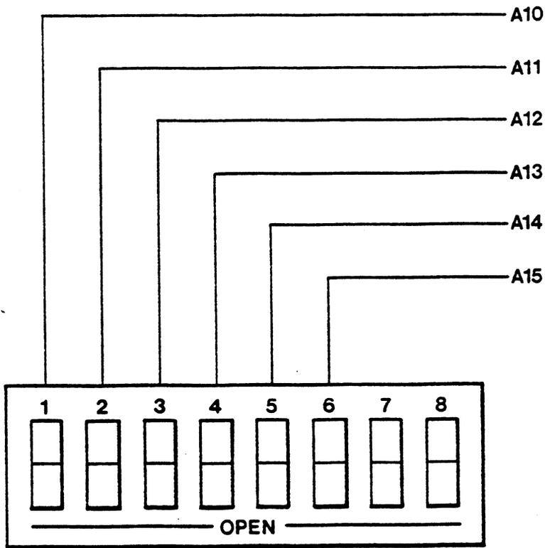
Figure 2-2. Switch Bank S2 - Base Address Switches
