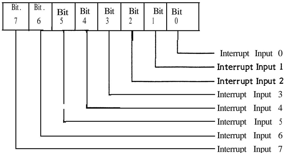
Figure 3-4. Interrupt Input Register
