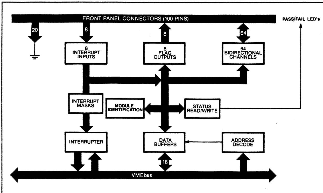
Figure 1-1. Operational Block Diagram of the DIO Module
