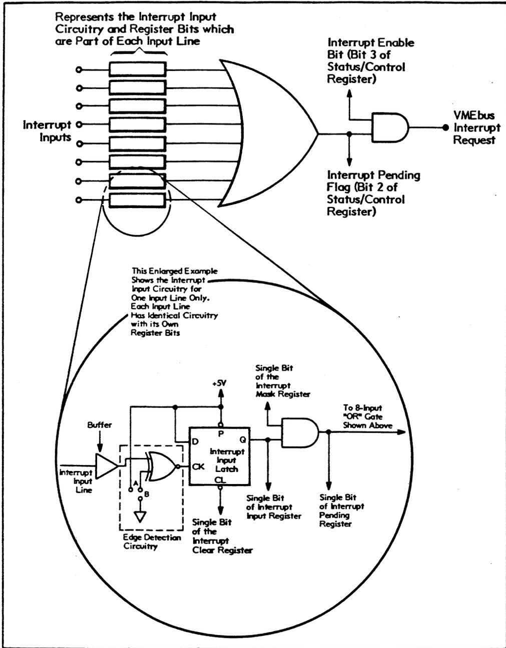
Figure 3-10. Interrupt Input Logic
